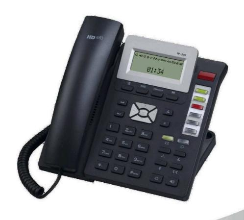
AppliedIP-200(P) is equipped with TI TITAN chipset and TI voice engine. It offers 2x15 characters LCD screen, 2 VoIP accounts, high-definition voice, and broad range of voice codecs. It has rich features including headset, PoE, PnP Autoprovision. In addition, IP-200(P) has 6 DSS keys, which could be programmed as the IP-PBX features like BLF/BLA, Call Completion, Call Recording, etc.
